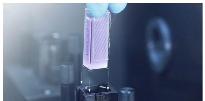
The holder positions the cuvette/filter in the light beam.
